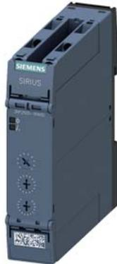
Timing relay, Multifunction 2 change-over contacts, 13 functions Positively driven Relay contacts 24...240 V AC/DC at 50/60 Hz AC 7 time ranges (0.05 s...100 h) with LED, Screw terminal
