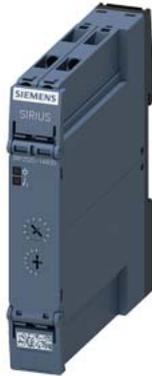
Timing relay, electronic on-delay 1 change-over contact, 7 time ranges 0.05 s...100 h 12-240 V AC/DC at 50/60 Hz AC with LED, screw terminal
