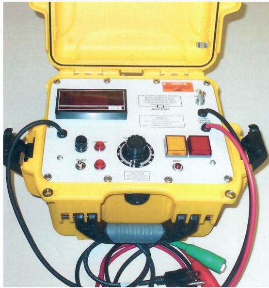
**Portable Dielectric Strength Tester (HI POT)
