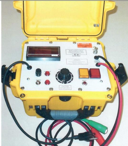
**Portable dielectric strength tester (Hi Pot)
