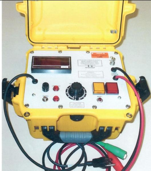
**Portable Dielectric Strength Tester (Hi Pot)
