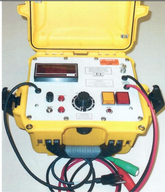
**Portable Dielectric Strength Tester (Hi Pot)
