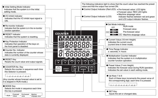
Note: Models with only 1-stage setting (H8BM-RAD/RBD) are not provided with pre-forecast and machine stoppage output function; only the forecast output function is provided.
