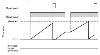
When the power supply is turned OFF, the display and outputs will turn OFF, but the current count/time value will be stored in internal memory.
