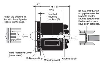
M 3×5 screws are used. Select solderless terminals referring to the figure below.
