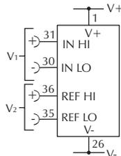
Measuring the ratio of two voltages.
