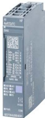
SIMATIC ET 200SP, Analog input module, AI 4xRTD/TC High Feature, suitable for BU type A0, A1, Color code CC00, channel diagnostics, 16 bit, +/-0.1%, 2-/3-/4-wire
