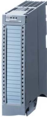
SIMATIC S7-1500 Analog output module AQ 4xU/I ST, 16 bit resolution, accuracy 0.3%. 4 channels in groups of 4; Diagnostics; Substitute value; Delivery including infeed element, shield bracket and shield terminal: Front connector (screw terminals or push-in) to be ordered separately
