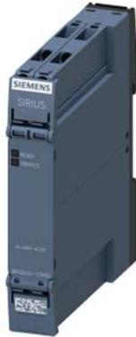
Thermistor motor protection relay Compact evaluation unit 17.5 mm enclosure Screw terminal 1 NO contact, 1 NC contact US = 24 V-240 V AC/DC Auto RESET suitable for bimetallic switch 2 LEDs (Ready/Tripped) galvanic isolation
