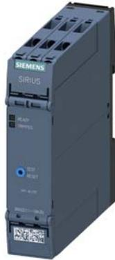
Thermistor motor protection relay Standard evaluation unit 22.5 mm enclosure screw terminal 2 change-over contacts US = 24 V AC/DC Manul/Remote-Reset with ATEX approval 2 LEDs (READY/TRIPPED) galvanic isolation Test/reset button Wire break monitoring Short circuit monitoring
