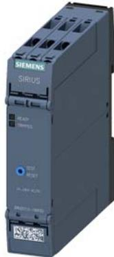
Thermistor motor protection relay Standard evaluation unit 22.5 mm enclosure screw terminal 2 change-over contacts US = 24 V-240 V AC/DC Manual/Auto/Remote reset with ATEX approval 2 LEDs (READY/TRIPPED) galvanic isolation Test/reset button Wire break monitoring Short circuit monitoring non-volatile
