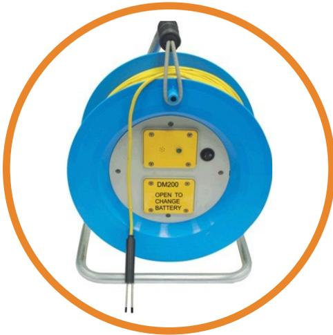
This is a simple but effective portable gauging system for determining the level of water in boreholes up to a maximum depth of 200 metres.
