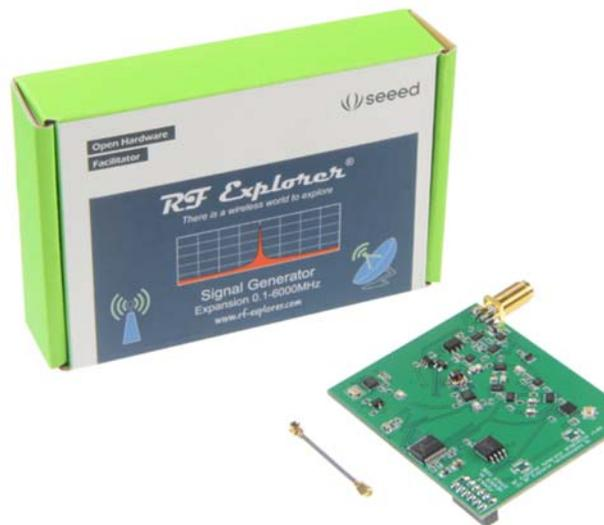
The Signal Generator baseline RFE6GEN can be enhanced to become a RF Explorer Signal Generator Combo. Full specifications are available in this article.
